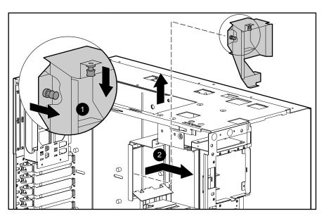
Figure 2-13. Removing the fan baffle
